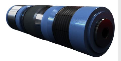
The Extended Reach Thermal Permanent Bridge Plug (ER-TPBP) is the thermal version of the reliable HM-18 and DB bridge plug. The thermal permanent bridge plugs are an economical way to suspend or abandon a well bore with casing deformation while maintaining the ability to drill out the bridge plug and re-enter the hole.
