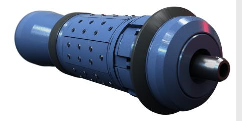
The ReacXion Slim Extended Range Dissolvable frac plug provides the performance of Steelhaus' standard ReacXion Complete plugs at a smaller running OD, allowing the plug to fit through tight restrictions without compromising pressure or temperature integrity. Conveyed via regular pump down operations, the plug can be set with conventional Baker style or equivalent setting tools. A proprietary coating allows the plug to be set in position hours prior to stimulation.
