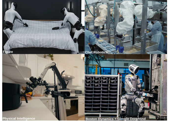
Fig. 1: Learned manipulation in four deployment settings. These are the organizations’ own published images and do not all correspond to the specific programs tabulated in Table XIII. Figure : two humanoids spreading a duvet, coordinated multi-robot, not single-robot bimanual, manipulation. Chef Robotics : hygienically sheathed arms portioning onto a moving conveyor, operators alongside. Physical Intelligence : a rail-mounted arm in an ordinary kitchen. Boston Dynamics and Google DeepMind : whole-body reaching at a parts rack on the Atlas platform. Panels reproduced from each organization’s public materials; copyright remains theirs.
