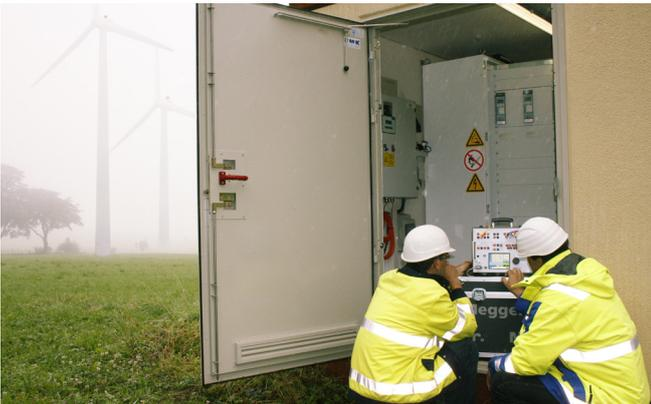
By helping detect and counteract islanding in distributed power generators, SVERKER 900's ramp instrument is useful to test frequency protection.
