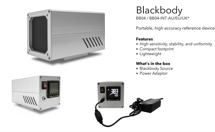
Our Blackbody has a fixed emissivity of 0.97 and is specifically designed to calibrate infrared temperature sensors. It was calibrated with a transfer standard at time of manufacture, which eliminates the need for offset. The emitting area is 2.75 inches (70 mm) square and features extremely high sensitivity, stability, and uniformity with an accuracy of ±0.1°C. Use it on any horizontal surface or with an optional tripod.
