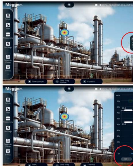
Tap the **○** on the top centre of the screen to view the **settings menu**. The menu can also be viewed by sliding the finger from the top of the screen downwards at any point.
