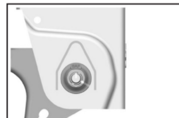
4. Marking for later visual inspection
