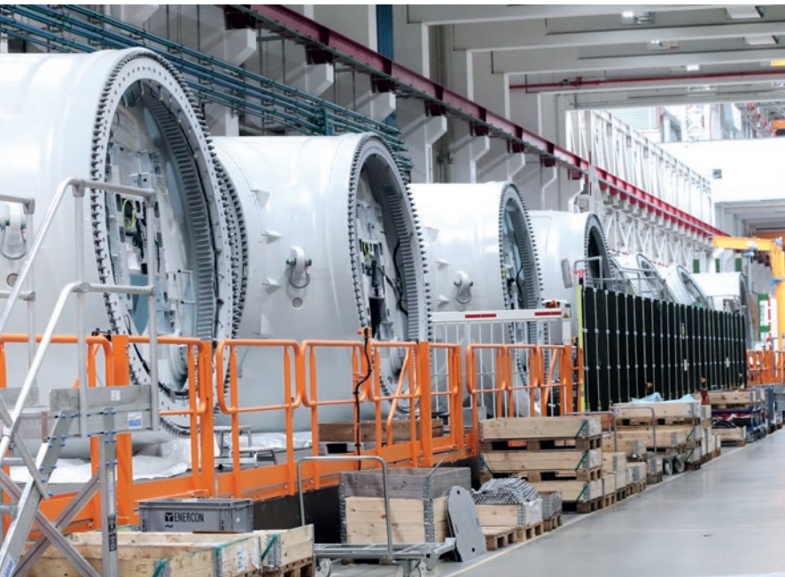
↑ A lean 'flow production' system has been set up on the hub production line.
