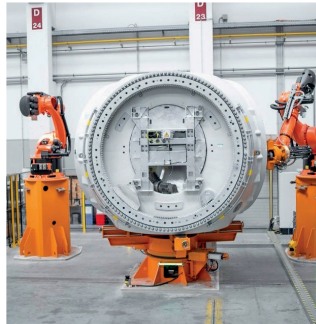
↑ Industrial robots carry out the time-consuming bolting of the bearings automatically.
