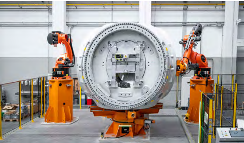
Automatic blade flange bolting system for hub production
