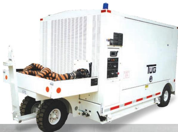
The TUG TMD Air Start is available in a 150, 180, 250, and 270 PPM.
