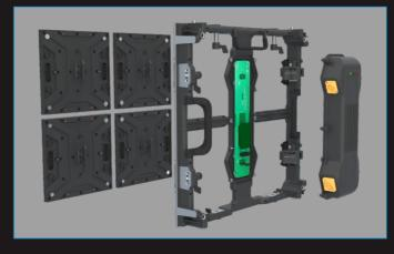
Modular design: Module, Power box and cabinet frame are three independent structures. Special module frame design ensures the flatness tolerance limit in 0.1mm.
