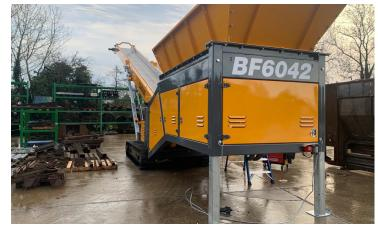
Cat 4.4 Power Unit, Tracked Bin Feeder 60ft x 42", 1200mm Wide Heavy Feeder and 1070mm Discharge Belt, Twin Drive on Feeder and Main Conveyor, Main Conveyor Lowers to Horizontal, 10m³ Hopper, Hyd Legs Under Feeder, Hyd Fold on Discharge, Galvanized Legs & Check Valves in Rams, (Fits in 45Ft HQ Container). Options: Dual Power, Fully Automatic Wireless Functions, Tipping Grid, Live Head, Hyd Auger, 1200mm Wide Discharge.
