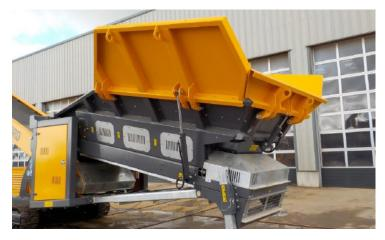
Cat 4.4 98kw Engine, Tracked Low Level Conveyor 80ft x 48", Twin Gearbox Drive, Twin Drive Discharge Belt, Cast Iron Pumps, Hyd Slew Hubs, Hyd Legs Under Feeder, Hyd Fold on Discharge, Galvanized Legs & Check Valves in Rams, 18m³ Hopper Capacity.
