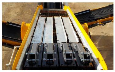
Barford SR124 Heavy Duty 3 Way Split Screen, 12' x 4'2" (3.66m x 1.28m) Screenbox, CAT 4.4 (56kw/75hp), 40" Heavy Feeder Belt, 40" Heavy Chevron Overs Belt, Impact System in Hopper, 42" Fines Collection Conveyor, Telescopic Extending Side Conveyors.
