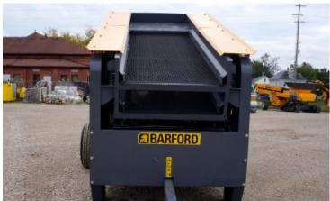
CAT 2.2 37kw Engine, Single Axle Mobile 12' X 4' (3m x 1.29m) Double Deck Screen c/w Extended Folding Fines Conveyor, Removable Towbar.
