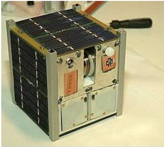
Ncube-2 , a Norwegian CubeSat (10 cm (3.9 in) cube)
