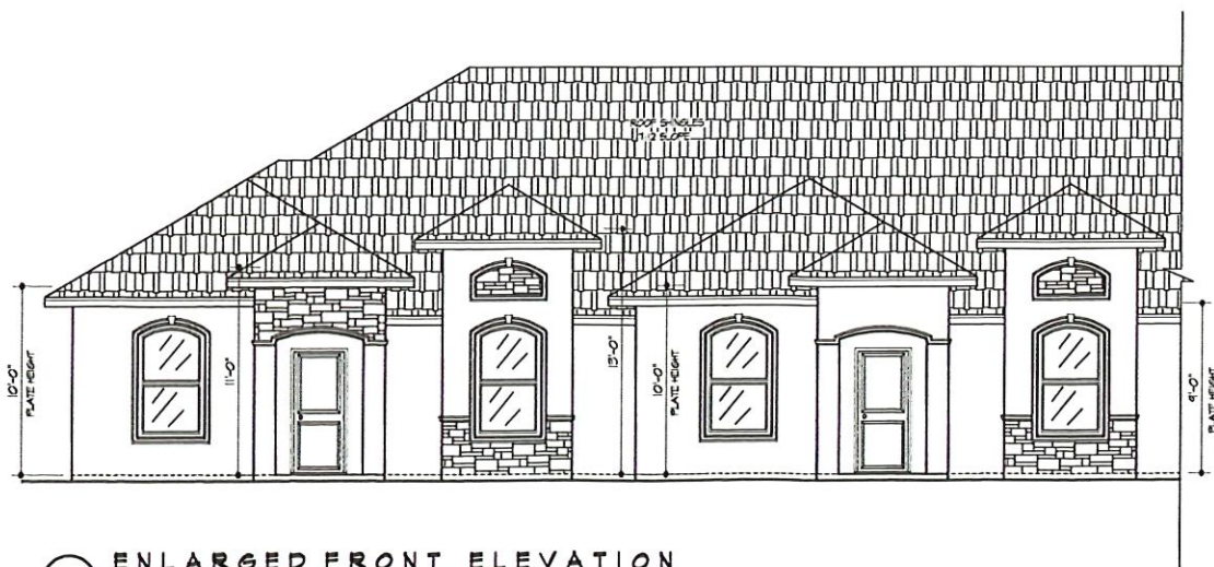
300 ENLARGED FRONT ELEVATION SCALE: 1" = 40'-0" REFER: 101 / A1.1
