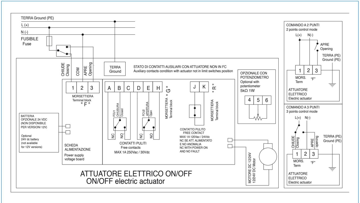
**SCHEMA ELETTRICO CON POSIZIONATORE DAL VB030 AL VB350 e DAL VB015M AL VB350M 12V AC/DC 50/60 Hz, 24V AC/DC 50/60 Hz, 100-240V AC 50/60 Hz**
