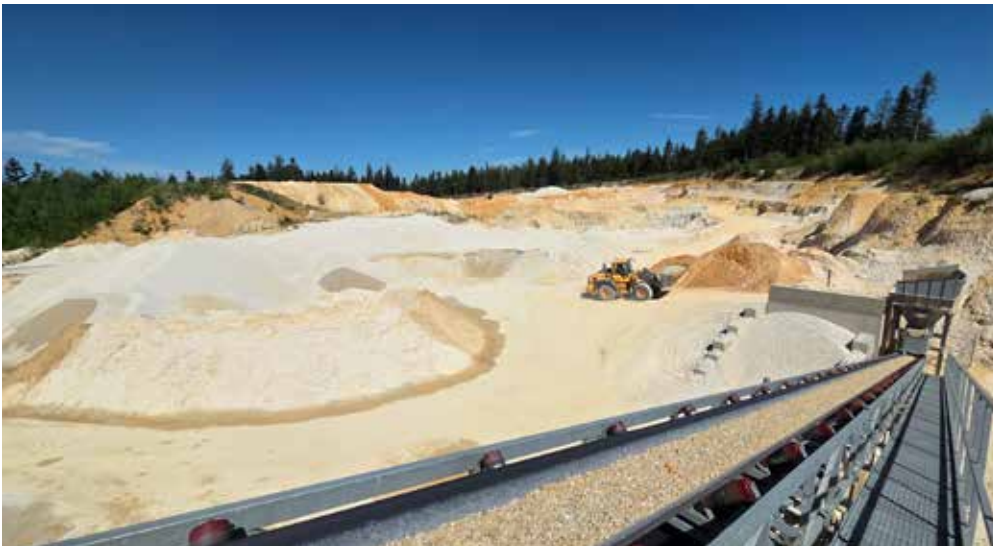
»3: Loosening and conveying the residual quartz gravel
