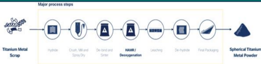
Figure 4: Simplified process flow diagram showing key process steps
