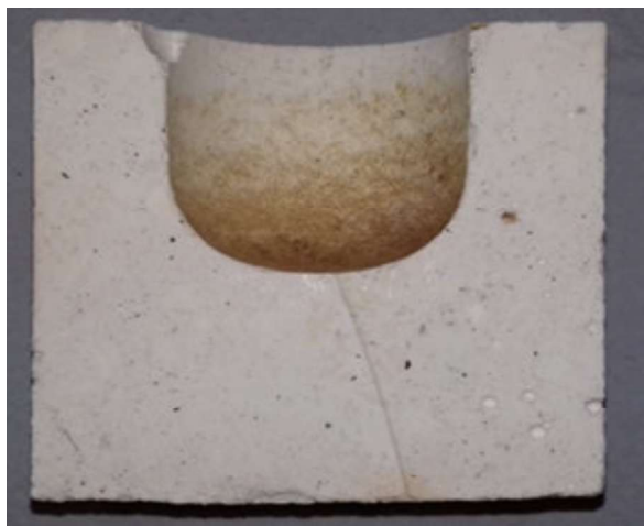
Fig. 3: Mill Scale Reaction test (1500°C)
