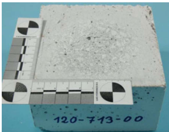
Fig. 2: Sample after hot abrasion testing
