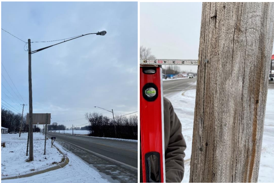
Figure 5-12: Measuring pole misalignment with a 4 ft. level
