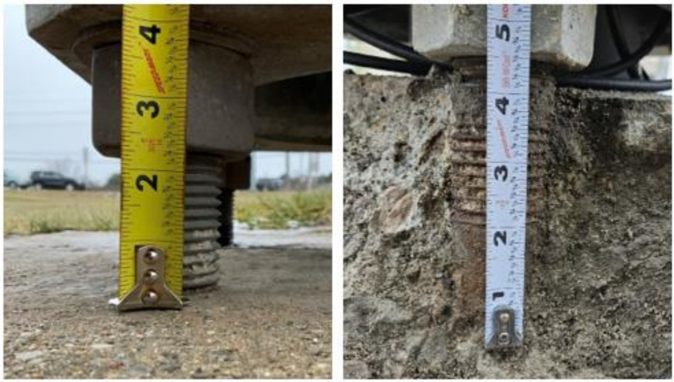
Figure 10-5: Standoff measurement for a sound foundation (left) and standoff measurement with foundation concrete deterioration (right)
