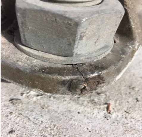
Figure 11-15: Non-frangible pole structure base plate crack
