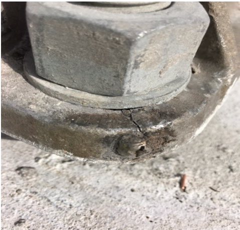
Figure 11-15: Non-frangible pole structure base plate crack
