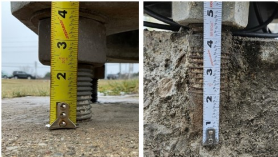
Figure 12-5: Standoff measurement for a sound foundation (left) and standoff measurement with foundation concrete deterioration (right)
