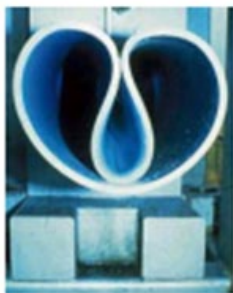
Figure 14: Deform-Reform Liner: "Heart" Shape of Folded HDPE Liner (left), Plastic Bands to Maintain the Shape (middle), and Coiled Pipe to Transport (right)
