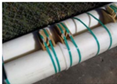
Figure 14: Deform-Reform Liner: "Heart" Shape of Folded HDPE Liner (left), Plastic Bands to Maintain the Shape (middle), and Coiled Pipe to Transport (right)
