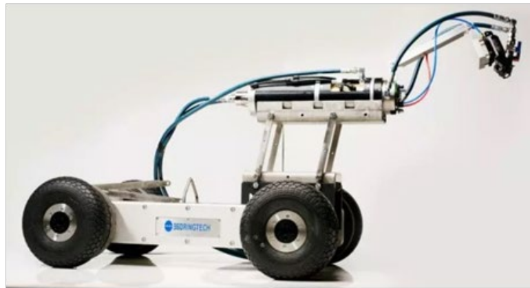
Figure 21: Sprayed-on Liners: Polyurea Coating Application (left) and Robotic Liner System (right)
