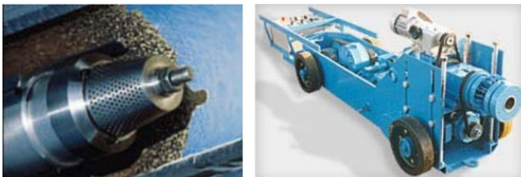
Figure 19: Spincast System Applies Material to Pipe Walls Using Centrifugal Force for Small Diameter Pipes (left) and for Large Diameter Pipes (right)
