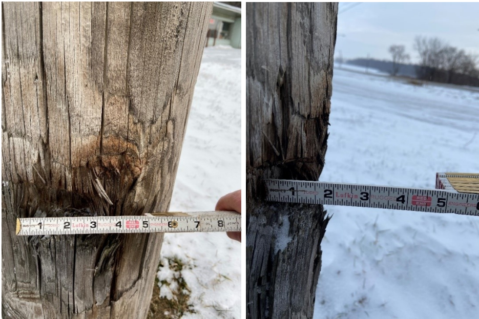
Figure 5-13: Measuring impact damage
