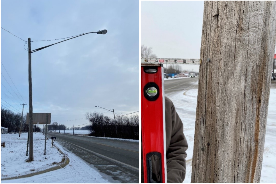
Figure 5-13: Measuring impact damage
