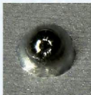
Cu-core solder ball
