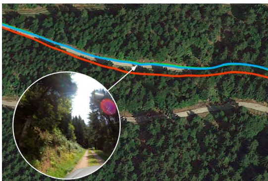
Figure 21 – Highlight 2 – along the east of the Black Forest route, shows S-GNSS ® OFF (red) away from the ground truth (green) with supporting image from a mounted video camera showing the true location. S-GNSS ® ON (blue) tracks the truth line closely.
