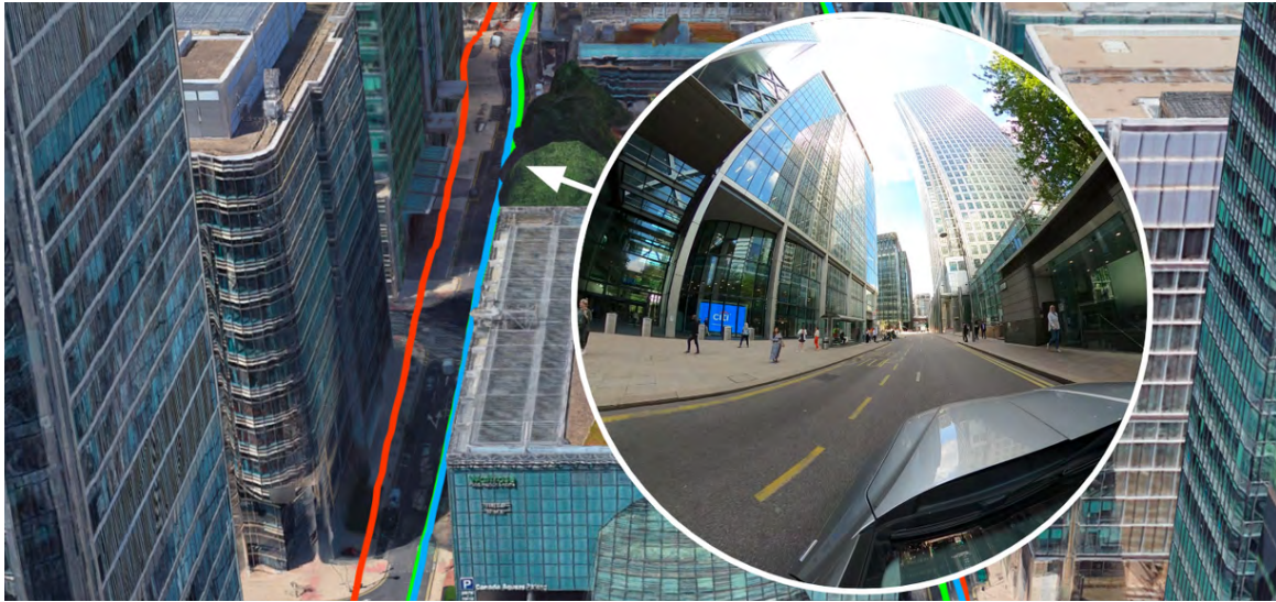
Figure 11 - View from east to west of Canary Wharf, showing S-GNSS® OFF (red) diverging away from the ground truth (green) with supporting image from a mounted video camera showing the true location (right hand lane). S-GNSS® ON (blue) tracks the truth line closely.
