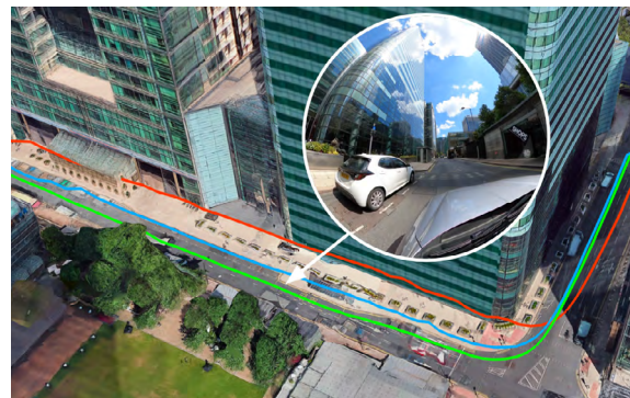
Figure 14 - View into the north of Canary Wharf, Lap 2, showing S-GNSS® OFF (red) away from the ground truth (green) with supporting images from a mounted video camera showing the true location (right hand lane). S-GNSS® ON (blue) tracks the truth line closely.
