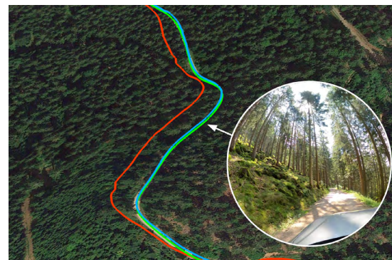
Figure 22 – Highlight 3 – along the south-east of the Black Forest route, showing S-GNSS ® OFF (red) away from the ground truth (green) with supporting image from a mounted video camera showing the true location. S-GNSS ® ON (blue) tracks the truth line closely.
