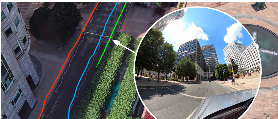
Figure 12 - View into the south west corner of Canary Wharf, Lap 1, showing S-GNSS® OFF (red) away from the ground truth (green) with supporting image from a mounted video camera showing the true location (right hand lane). S-GNSS® ON (blue) tracks the truth line closely.
