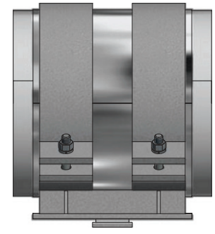
DOUBLE CLAMP = +/- 4-1/2" AXIAL MOVEMENT - WITH GUIDES
