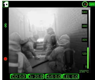
Example: Grayscale Mode with 3rd Party Gas Detector Link via BLE
