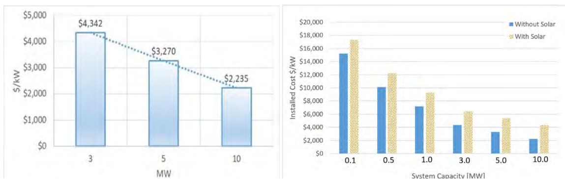
Figure 2: (Left): Estimated capital costs for h-mcs-PSH systems per kW installed for 3, 5 and 10 MW systems, not including renewable component. (Right): Estimated installed system costs with and without solar panels, for system capacities ranging between 100 kW to 10 MW. The cost of the solar panels was based on generation occurring during periods of sunshine at the system capacity (MW).
