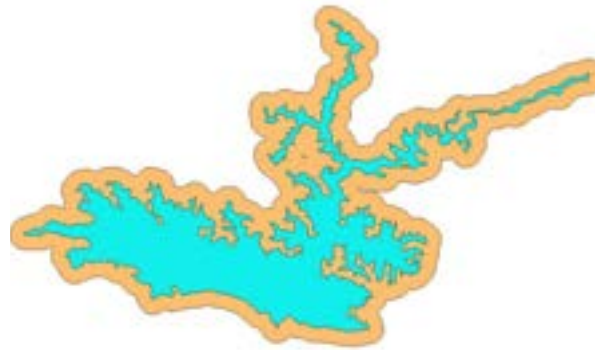
Figure 2: Example of impounded area land cover using the buffer method, the turquoise area representing the reservoir surface area and the orange stripe the 25% of the equivalent spherical diameter. It is calculated as:
