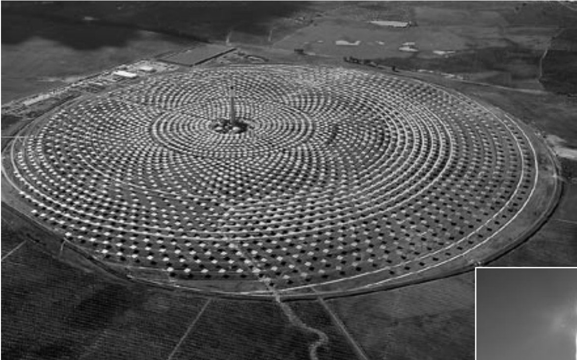
In Spain, the Gemasolar 19.9 MW solar-thermal power plant, with molten salt storage, has achieved 24 hours of uninterrupted electricity production. If Spain can do it, Australia can too!
