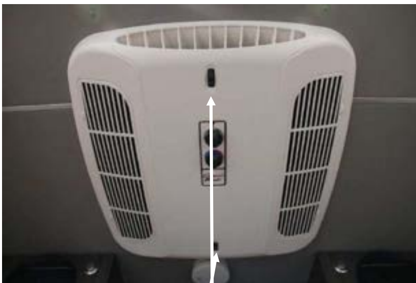
Air output controls PHOTO F-10
