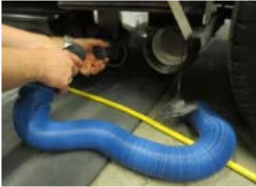
Dumping station connection PHOTO D-36
