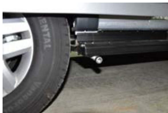
Furnace exhaust outside vehicle
