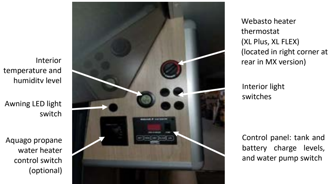
Controls PHOTO A-3
