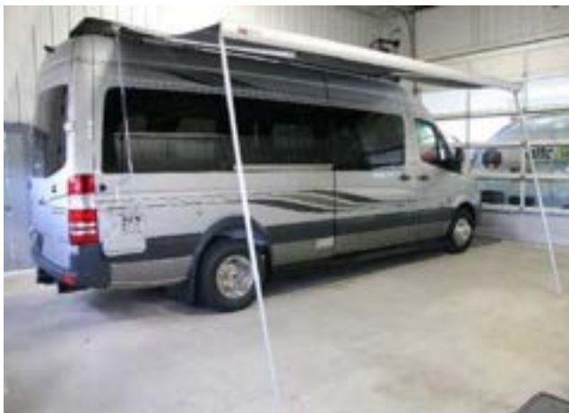
Vertical supports at an angle PHOTO F-17
