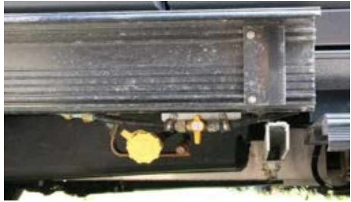
Running board propane valves, driver side (MX)
