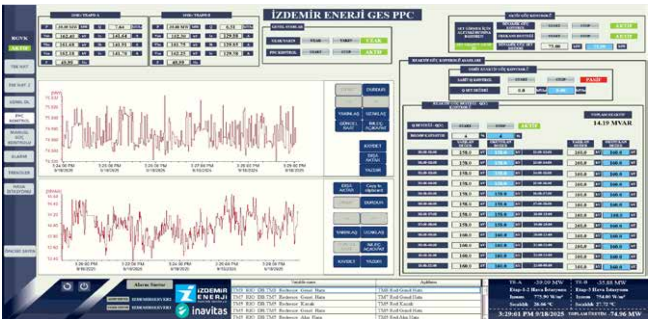
The dashboard shows İzdemir's PPC in action, aggregating data across grid systems, monitoring power trends, and enabling centralized operator oversight through a single interface.
