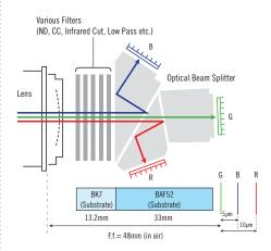
Specifications for the interface between the lens and a 2/3" HD CCD camera.
