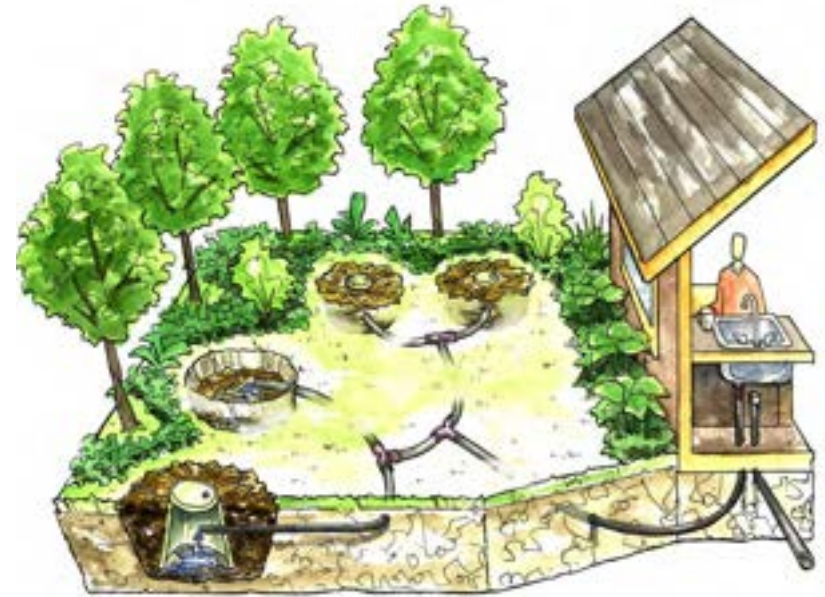
A branched greywater system irrigates trees from the kitchen sink.
