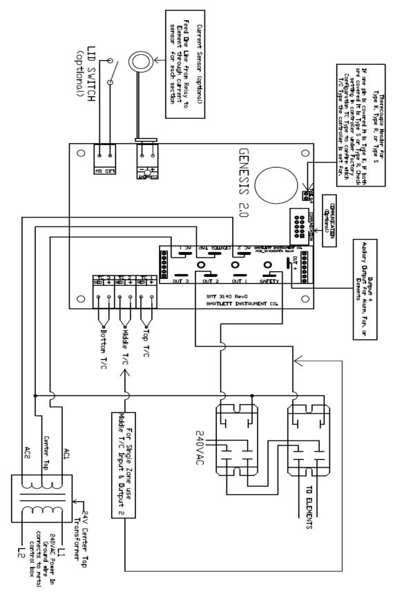
GENESIS 2,0 WIRING DIAGRAM WITH 1/4 Inch QUICK CONNECT ADAPTER BOARD
