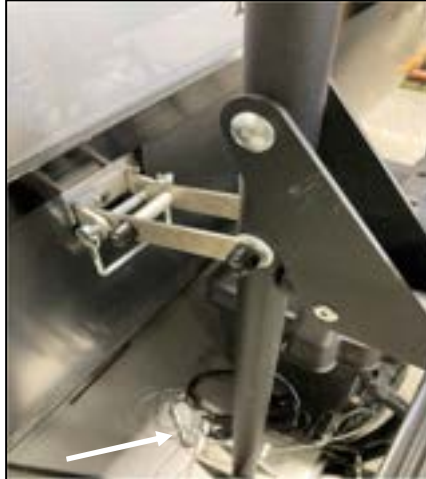
PHOTO K-30 Bolts and pins to install bike rack
