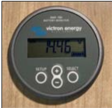
PHOTO I-2 Lithium battery monitor
