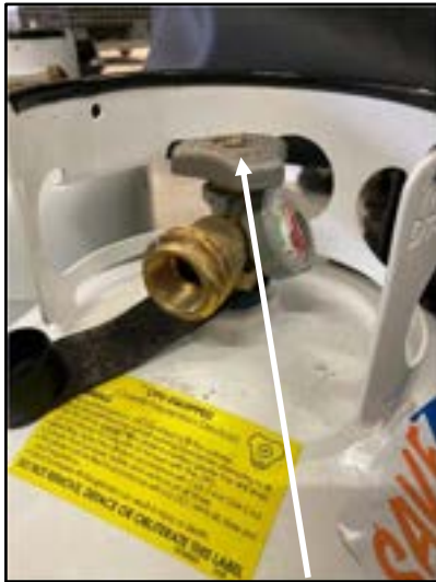
PHOTO G-1 Propane tank valve and tap
