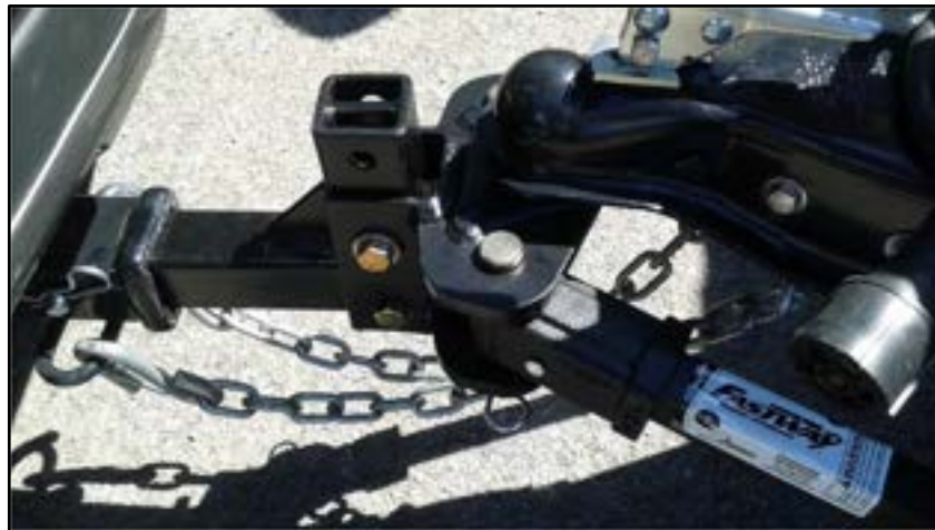
PHOTO M-4 Safety chains
