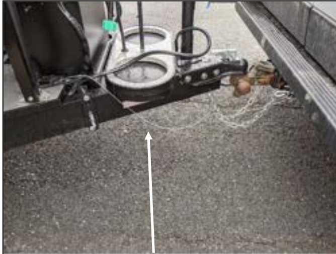
PHOTO M-1 Breakaway switch cable loop
