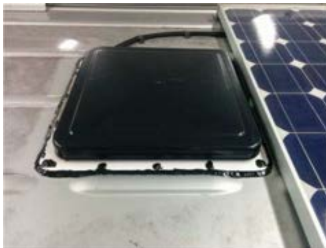
Roof vent gasket PHOTO G-1
