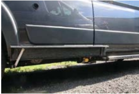
Running board propane valves, passenger side (XL Plus and XL FLEX)
