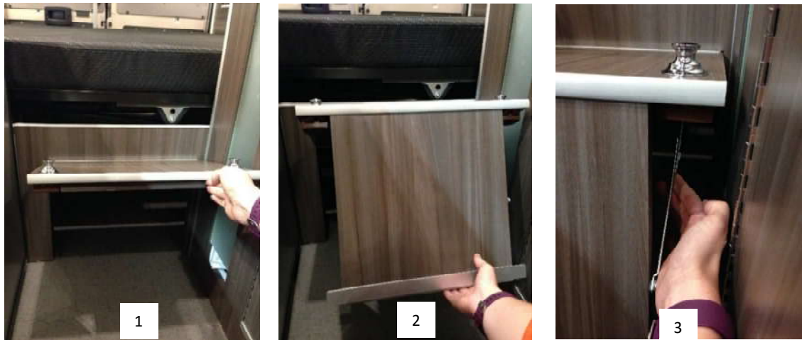
Installation of step to access adjustable bed
