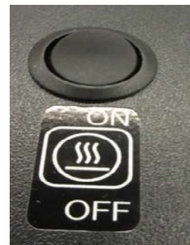
Front heater switch
