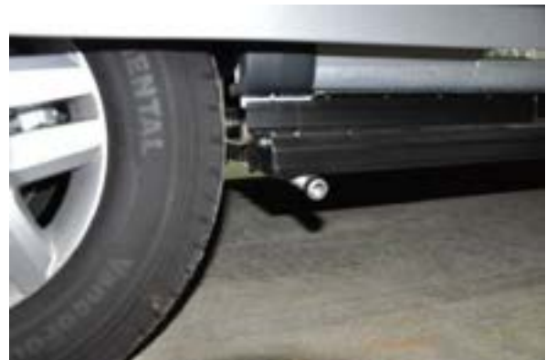
Furnace exhaust outside vehicle
