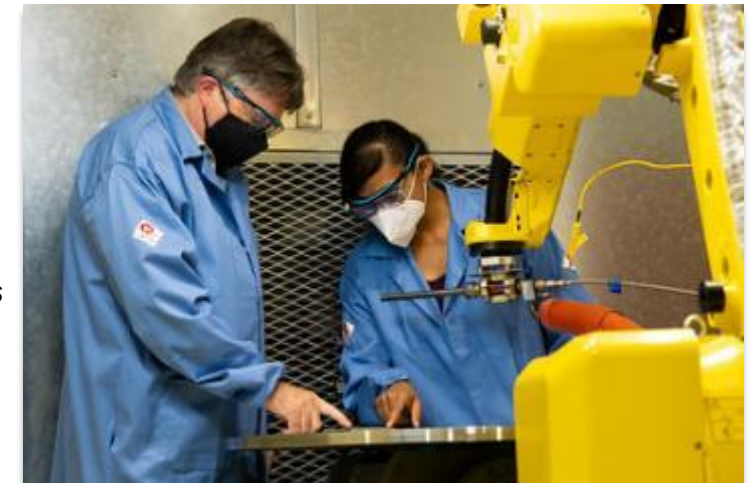
Photo: Prepping cold spray repaired coupons for cavitation testing. Credit: Andrea Starr, Pacific Northwest National Laboratory
