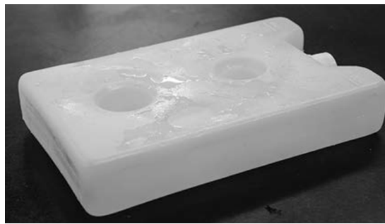
Fig. 2.25 Condensation on a conditioned water pack
