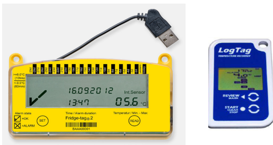
Fig 2.13 30-day electronic temperature recorders
