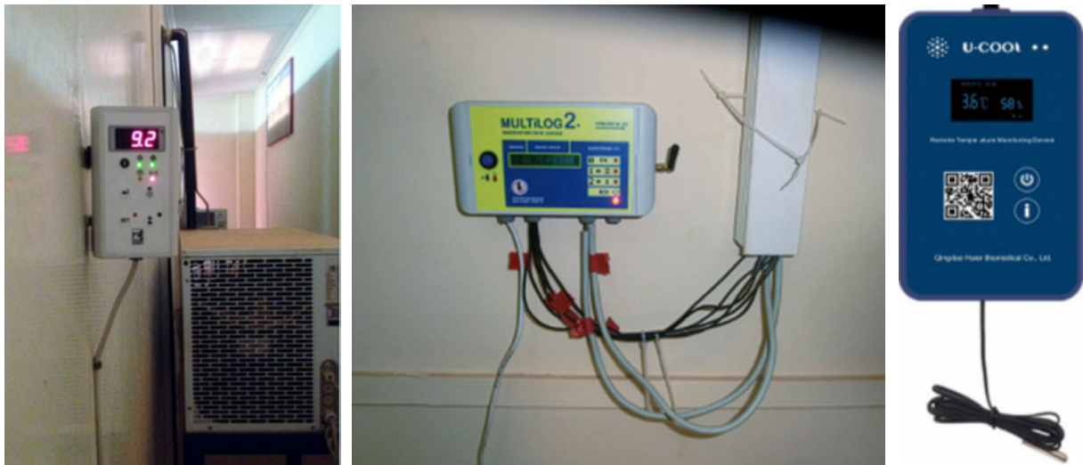
Fig. 2.16 Remote temperature-monitoring devices
