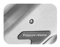
All pressing operation will stop and piston rod will retract to full open position.
