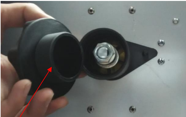
(1) Remove the spool retaining nut.
