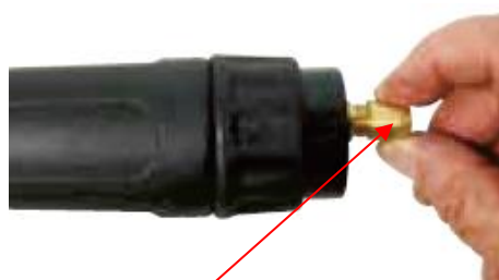
(6) Fit the liner retaining nut and screw only 1/2 way down.
