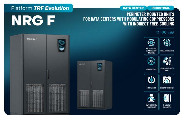
NRG F units are water-condensed perimeter-mounted cabinets that are able to exploit the **effect of indirect water-based Free-Cooling**. The F Series uses Dry Cooler water as both a cooling source for free-cooling and a heat exchange fluid for condensing the cooling circuit. NRG F units are "monobloc" units inside which the **entire cooling circuit** is concentrated. Cooling is via a **brazed plate exchanger made of stainless steel AISI 304.**
