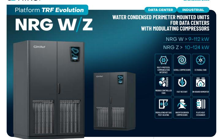
The NRG W units are water-condensed perimeter cabinets. The W series uses Dry Cooler water, the Z series on the other hand uses low temperature mains water or groundwater (15°C). The NRG units of these series are monobloc units inside which the entire cooling circuit is concentrated, cooling is via a brazed plate exchanger made from stainless steel AISI 304.
