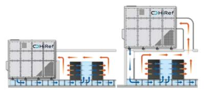
Example of use for a 1 MW Data Center (Redundancy N+1) in Amsterdam at  $36^{\circ}$ C -25%; Air temp.  $24^{\circ}$ C; Max air temp. in  $26^{\circ}$ C
