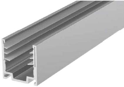
High-quality 6063 aluminum with thin-wall, light-weight design. Includes a serrated silicone grip insert designed to hold fixture with additional force. Recommended on projects mounted upside down. It is deformation and rust resistant, and cost-effective. Please refer to install manual for proper installation practices.
